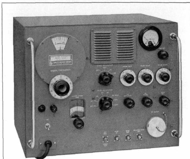
Fig. 1. New -hp- Model 626A SHF Signal Generator has high power output over 10 to 15.5 kmc range, is provided with direct-reading frequency dial and output attenuator, has flexible modulator.
